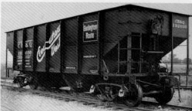
The first HT-5A, Q 192600, at Galesburg in August 1940 with the "Everywhere West" stencilling which by then was standard. This car and 192008 at left both ride on National Type B trucks.—CB&Q photo, Rod Masterson collection
