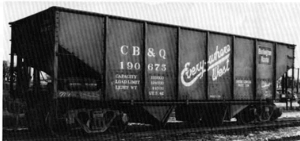
CB&Q HT-1 190137, one of the original 1926 AC&F cars, displays a post-1937 paint scheme in this 1940's view at Omaha. The horizontal seam in the side panels is readily evident.—Bernard Corbin photo, BRHS collection
