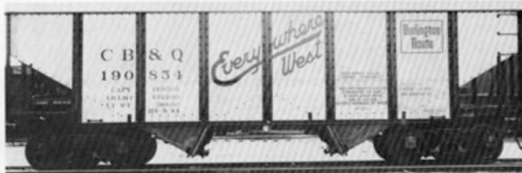
HT-2 190854 was retrofitted with aluminum side, end and slope sheets at Havelock and photographed there on Aug. 11, 1944, upon completion of the work. Note that two-piece side panels were still utilized.—CB&Q photos, Rod Masterson collection
