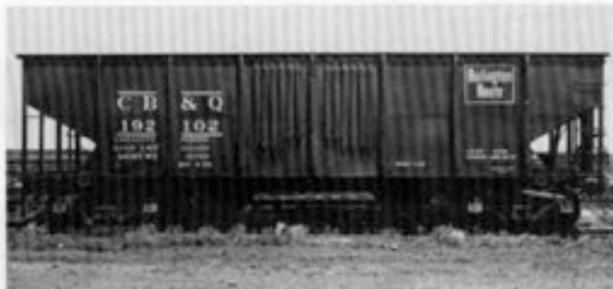
The 189000-series HT-5B's were extensively overhauled at Havelock in 1959 and thereafter wore the "new image" Chinese red paint scheme, including black trucks. Few other Q twin hoppers received the Chinese red scheme. Havelock, March 11, 1959.—CB&Q photo, Rod Masterson collection
