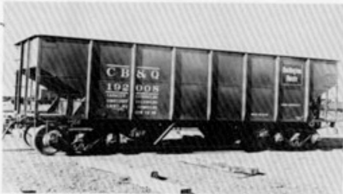
Ninth of the "new design HT-5's, Q 192008 posed fresh from the steel car shop at Galesburg in December 1936. These were the final cars delivered without the "Everywhere West" stencilling.—CB&Q photo, Rod Masterson collection
