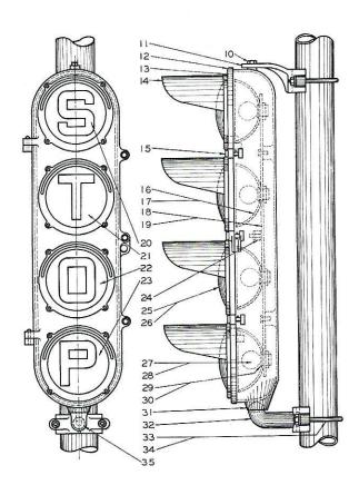
The Type 2800 Illuminated STOP Unit is equipped with bayonet base lamp sockets whereas the Type 2801 Unit is furnished for use with medium screw base lamps. Bayonet base lamp sockets are single contact.
